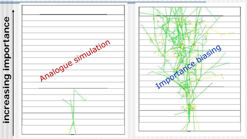
10 MeV neutron in thick concrete cylinder
