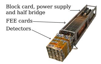
Block is mounted on a copper base in which water flows to provide cooling
