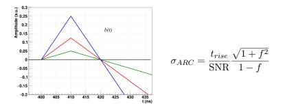
Zero crossing of the bipolar signal  $b(t) = f \cdot s(t) - s(t - t_D)$
