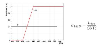
Intersection between a fixed threshold T and the signal s(t)
