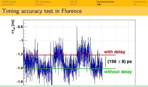
Expected  $(t - t_{ref})_{del} - (t - t_{ref})_0 = t_{del} \simeq 207 \text{ ps}$ GOOD AGREEMENT
