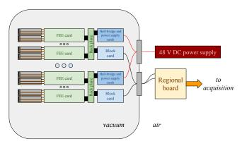
up to 36 block cards are connected to a regional board via a full duplex 3 Gb/s optical link
