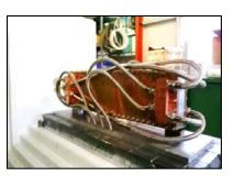
Up to **500 μA** current and **70 MeV** energy proton beam (**35 kW**) delivered to the high power Beam Dump Less than 1% beam loss
