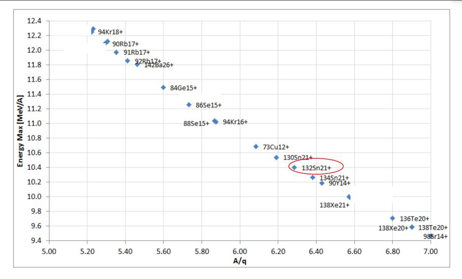
Energy from SPES Post-Accelerator as function of A/q
