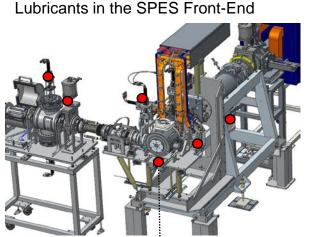
TIS handling Lubricated bearings Integrated dose ≈ **30 MGy** in **7 y CRITIC COMPONENT**  [1] PRODUCTS SELECTION ✓ 9 products
