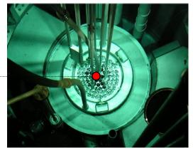
Central Thimble irradiation facility TRIGA MARK II Research Reactor
