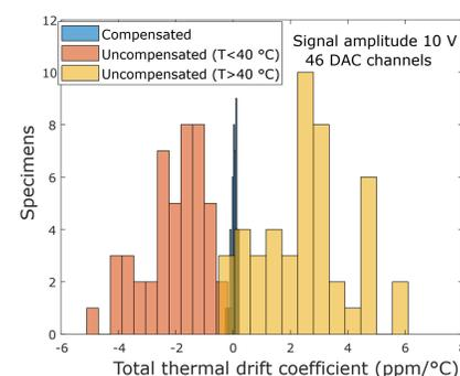
Figure 8: Pulse amplitude thermal drift coefficient before and after calibration
