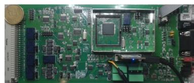
Figure 7: Photograph of a 4 channel pulser board. Each channel is connected to several heaters in parallel
