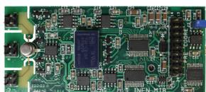
Figure 5: Photograph of the preamplifier
