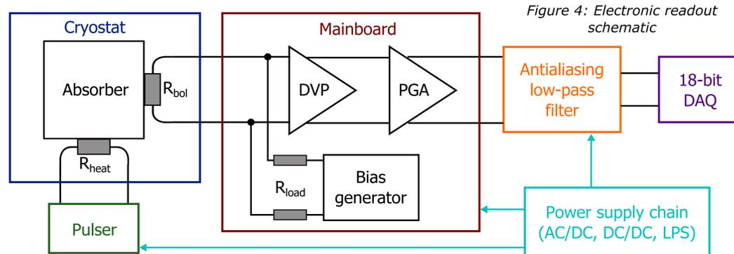
Figure 4: Electronic readout schematic
