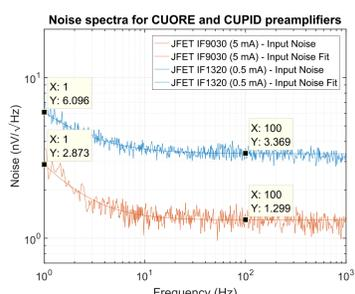
Figure 6: Input voltage noise of CUORE (blue) and CUPID (red) preamplifiers
