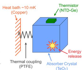
Figure 3: Schematic picture of a bolometric detector
