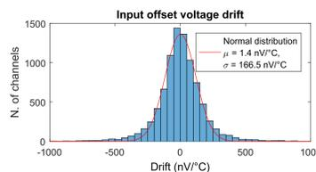
Figure 10: Input offset voltage drift for all channels
