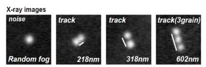
Nuclear emulsion: AgBr crystal (40nm) and organic gelatine Readout system: Optical Microscope Threshold: 100 nm track length
