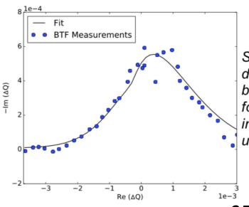
Stability diagrams have been measured for the first time in the LHC by using BTFs
