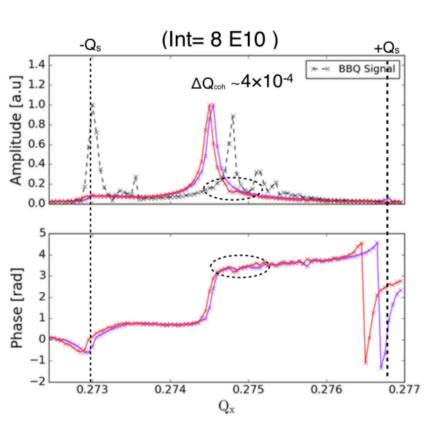
Collective effects change the beam response and makes it very difficult to reconstruct the Stability Diagram by using an analytical fitting function.
