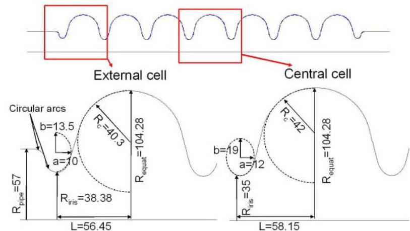
Figure 1: cavity profile and dimensions.
