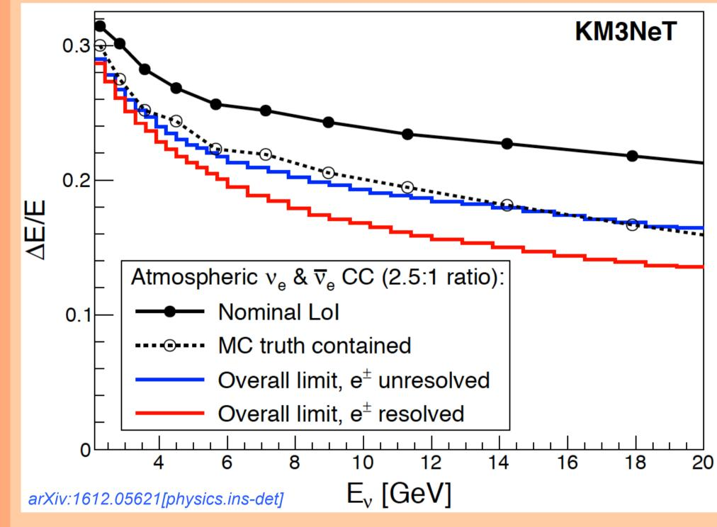
Resolutions for ORCA detector with 6m vertical spacing between DOMs
