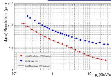
Resolution of transverse plane impact parameter for **current** and **upgraded** ITS<sup>[5]</sup> (fast and full MC simulation results shown)
