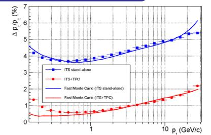
Transverse momentum resolution for the upgraded ITS, in particular for **ITS stand-alone** and **ITS-TPC combined**<sup>[5]</sup> (fast and full MC simulation results shown)
