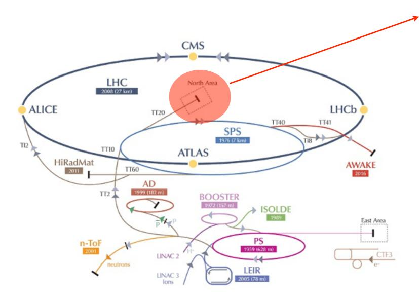
In the North Area the SpS extraction line is providing a secondary charged hadron beam
