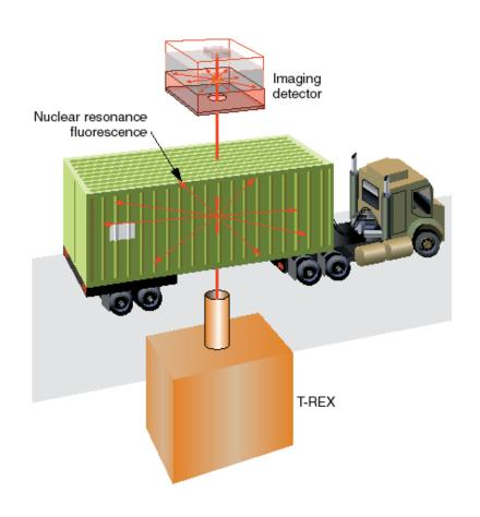
Detection of special nuclear materials Non-destructive interrogation If positive signal: identification 10 seconds per cargo container
