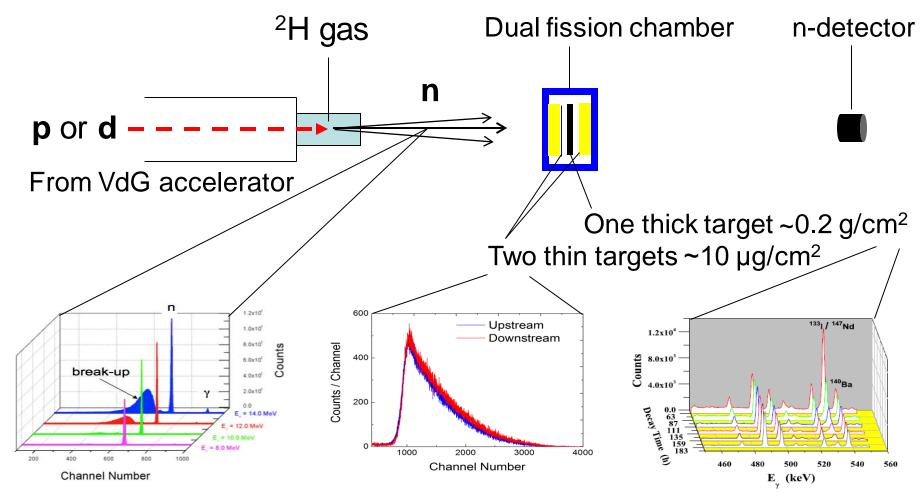
(Gamma\_count / Fission\_count) = (m<sub>thick</sub> / m<sub>thin</sub>) \* FPY \* C
