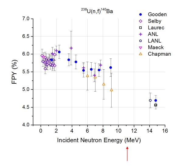
9 MeV datum not corrected for off-energy neutrons from <sup>2</sup>H(d,n)<sup>3</sup>He reaction
