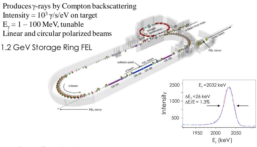
Beam time structure: Rep rate = 5.58 MHz (T = 180 ns) and  $\Delta t$  = 100 ps
