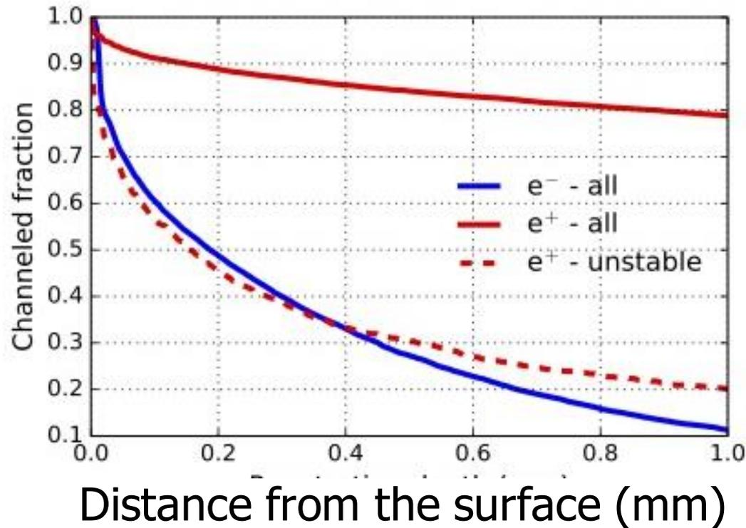
Simulation of electron and positron dynamics in the crystal via DYNECHARM++
