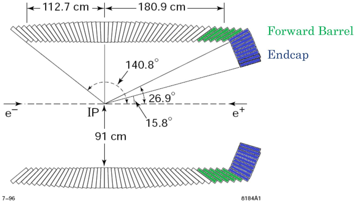
**Figure 3-11.** The EMC layout: Side view showing dimensions (in mm) of the calorimeter barrel and forward endcap.
