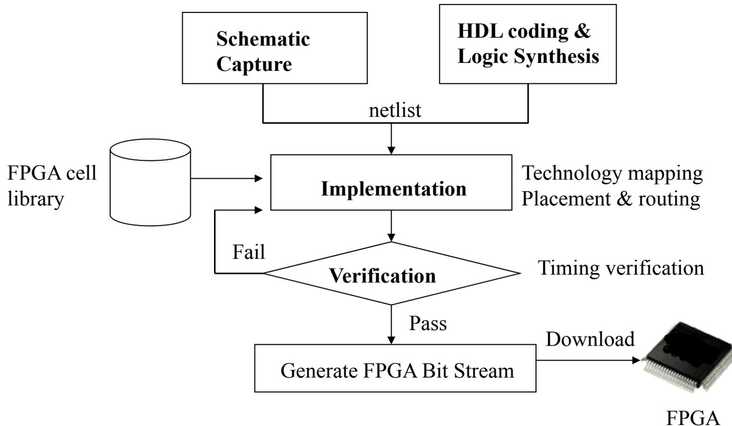
**THIS APPROACH HAS EXTREMELY FAST TURN-OUT TIME SINCE THE FPGA DEVICES HAS BEEN ALREADY FABRICATED**
