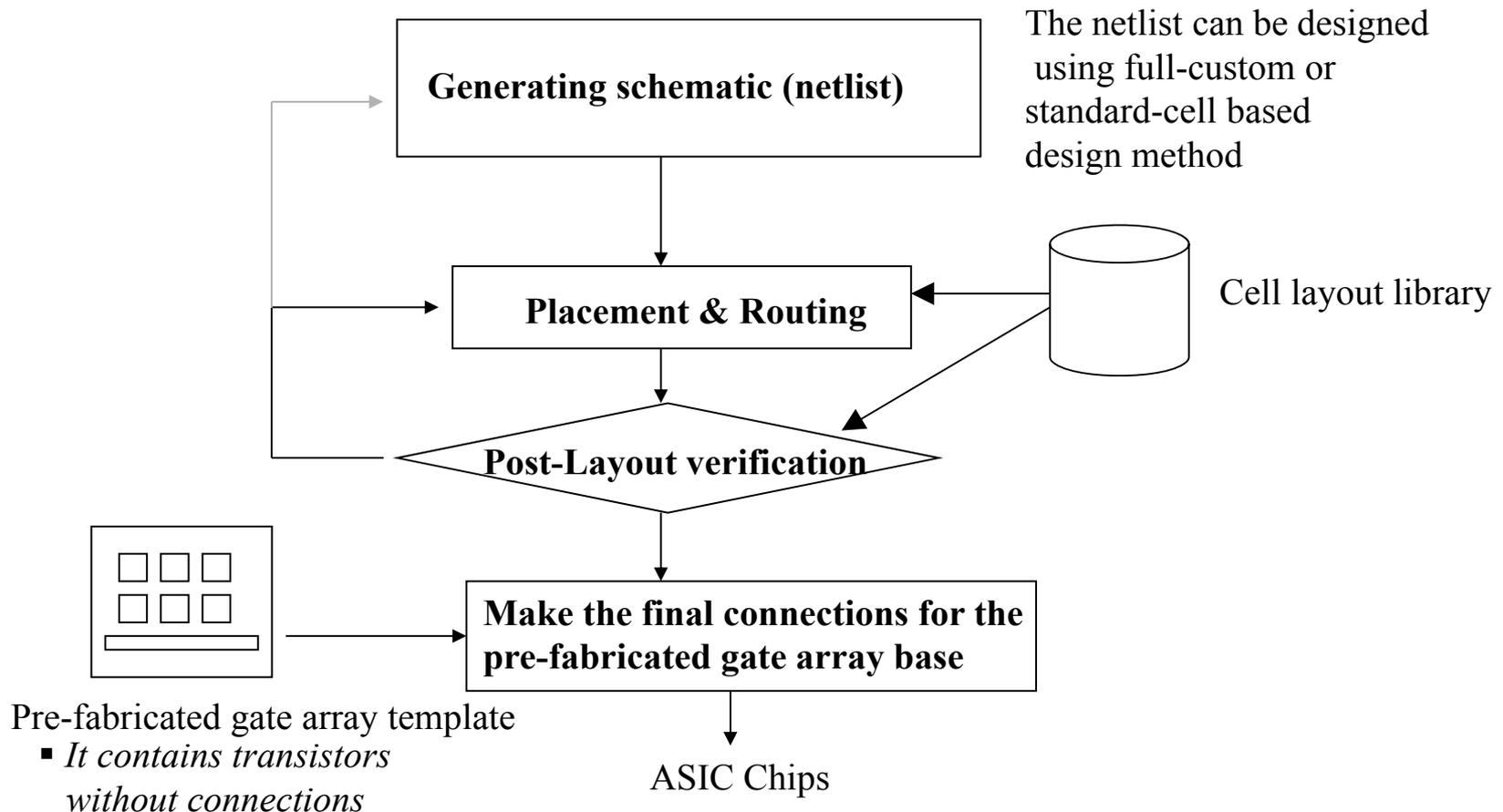
**FASTER THAN THE STANDARD-CELLS BASED APPROACH AS PART OF THE FABRICATION PROCESS HAS BEEN DONE**
