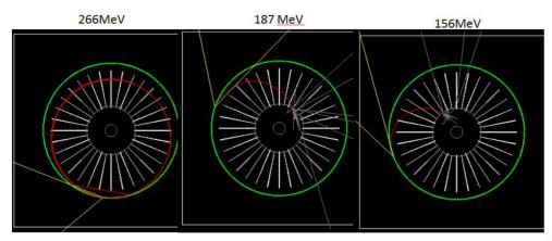
**Figure 6:** Example positron trajectories in the detector system at three different energies of positrons. The green circle is the muon beam orbit. The red trajectory is the trace of the positron track. The white tracks are photons.
