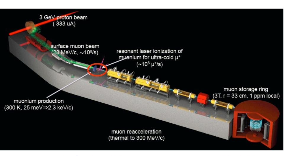
Injection of an ultra-cold, low-energy, muon beam into a small, but highly uniform magnet
