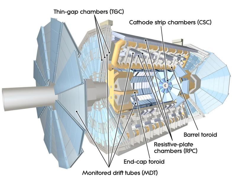
Multiple layers of tracking and trigger chambers that cover  $|\eta| < 2.4$
