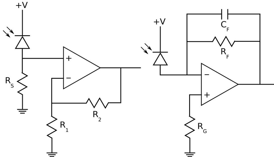
In voltage amplifiers increasing  $R_S$  increases input amplifier voltage, but amplifier input voltage noise increase and bandwidth decreases.
