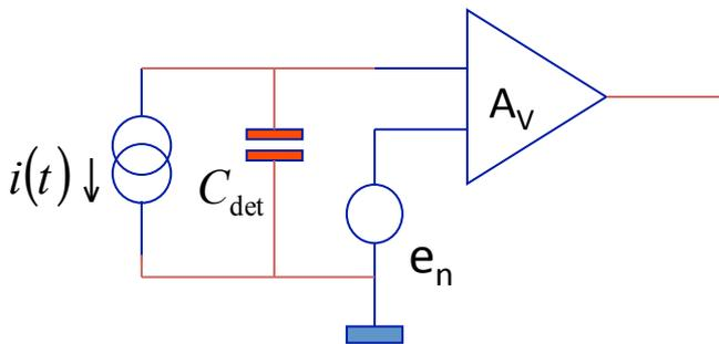
$$V_{out} = \frac{Q_{in}}{C_{tot}} \quad C_{tot} = C_{det} + C_{conn} + C_{in\_pre}$$
