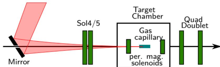
Figure 1: Setup for external injection in a laser-plasma wakefield
