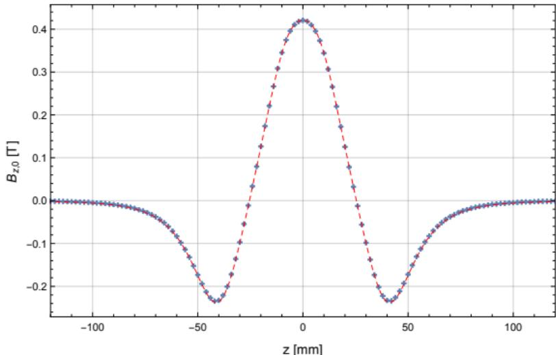
Figure 3: Long. field profile - measured and simulated.
