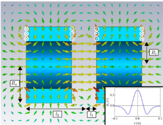
Figure 2: CST simulation and long. on-axis field  $B_z$ .
