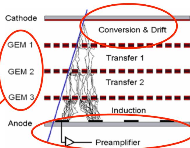
Working with different levels of gain it is possible to obtain high level of gamma-neutron discrimination
