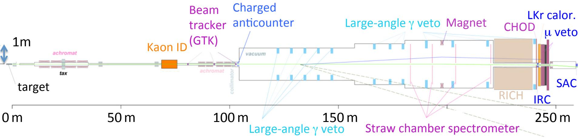
Can track 750 MHz beam ( $6\% K^+$ ) and sustain  $\sim 5$  MHz  $K^+$  decay in a **60-m long volume in vacuum**
