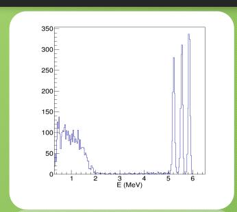
To measure the detection threshold, we have performed a run using a standard 3-peak alpha source and a americium source shielded by a 17 µm thick Al foil. This degrader shifts the energy peak to 1 MeV and, due to energy straggling, the energy range spanned reached zero.
