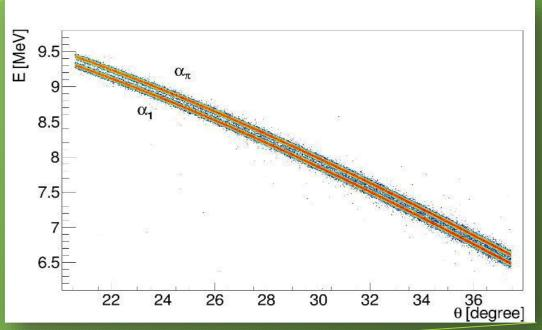
The simulation takes into account the energy and position resolution considering beam energy spread, target thickness and detector resolution.
