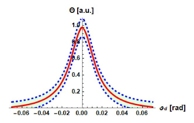
Angular distribution of the electron beam detected inside the bubble (red curve). The blue dashed curves delimit the error region (light green-shadowed). Beam rms divergence 13±2 mrad.
