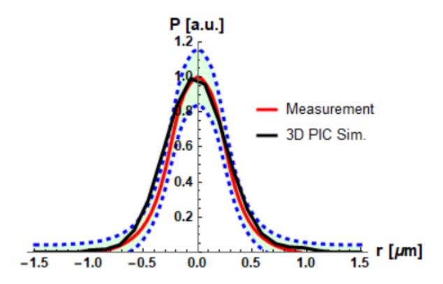
Electron beam radial profile detected (red curve) and simulated (black curve). The blue dashed curves delimit the error region (light green-shadowed).
