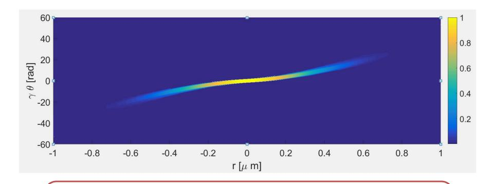
$$\epsilon_{r_{\beta}N} = \gamma_0 \sqrt{(\sigma_{\gamma}/\gamma_0)^2 \sigma_r^2 \sigma_{\theta}^2 + \epsilon_{r_{\beta}}^2}$$
