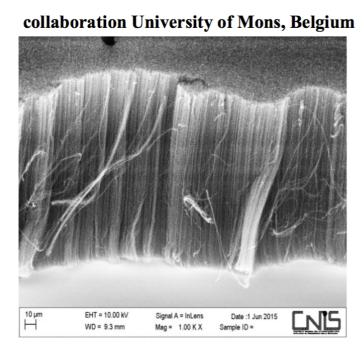
length: 100  $\mu$ m (can be increased) ext. diameter: (20 ± 4) nm aspect ratio:  $5x10^4$
