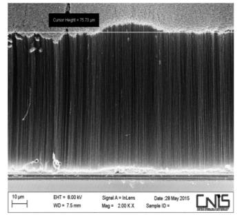
length: 75  $\mu m$ ext. diameter: (13 ± 4) nm aspect ratio: 0.6 x10<sup>4</sup>
