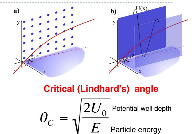
If  $\theta < \theta_{C}$  ions are channeled!  $\theta_{C} \sim 4 \text{ deg}$  for <sup>6</sup>C channeling
