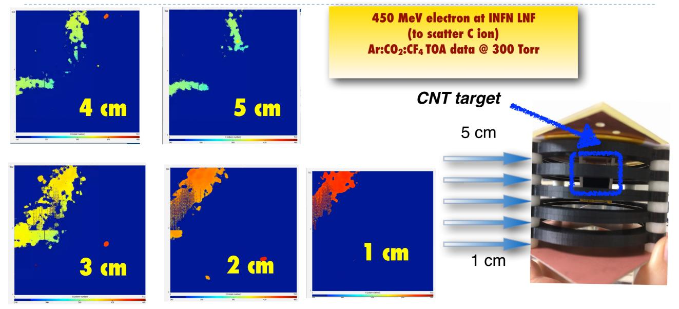
Color is drift time (along Z) for different Z position (X-Y projection)
