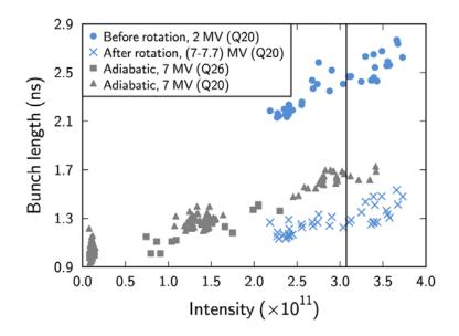
Bunch length (4 sigma Gaussian fit) achieved adiabatically or using bunch rotation
