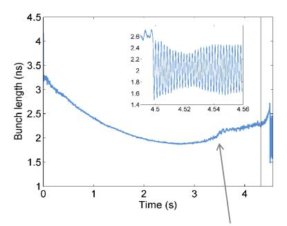
Bunch length increase due to uncontrolled emittance blow-up
