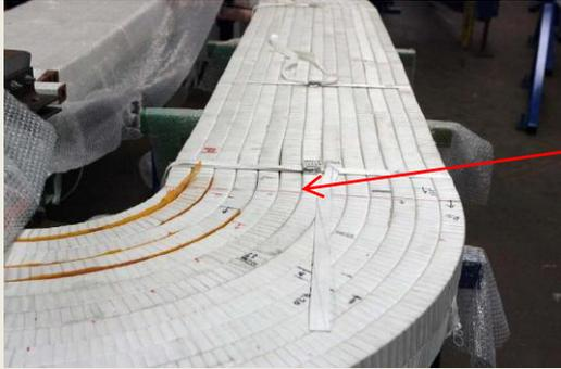
The conductor xsect is 1"x1". Initially, winding even this simple race-track design without warping was a challenge.
