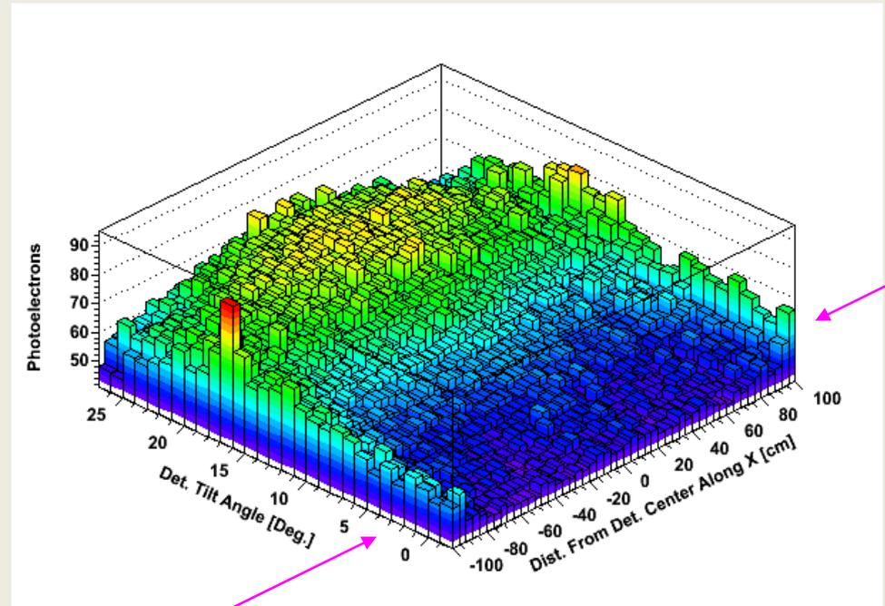
When the bars are oriented close to a vertical plane, the uniformity is optimized. This is important.
