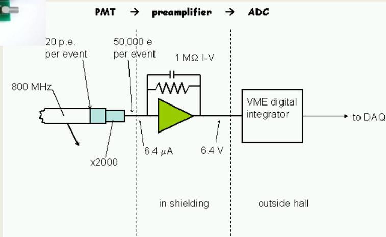
Electronic noise is over two orders of magnitude smaller than counting statistics noise of electron tracks.
