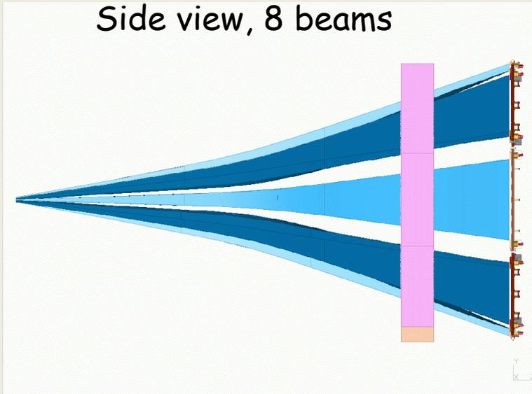
The design required apertures for 8 beam envelopes large enough to provide some shielding while doing no harm (i.e., minimal showers from scraping)
