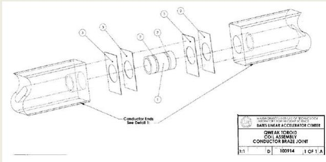
Occasionally, the conductor has to be spliced. A tough bit of plumbing. Without good quality control in the brazing, the joints would leak when warm and pressurized.
