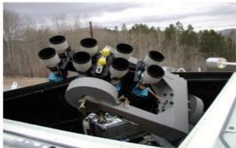
The RAPTOR-P telescope has a 500 sq-degree field-of-view and can simultaneously cover the full LIGO and Fermi boxes for early optical emission starting about 6 seconds after the receipt of event trigger.
