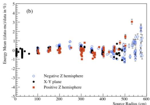
Energy reconstruction algorithm improved by inclusion of scattered and reflected Čerenkov light. Validated by extensive comparison of calibration data and simulated data. Calibration sources: Laser,  $^{16}\text{N}$ ,  $^8\text{Li}$ ,  $^{252}\text{Cf}$ , Am-Be, cosmogenic neutrons, etc.
