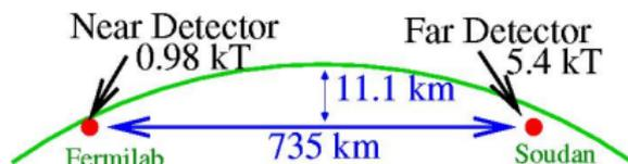
A  $\sim 3$  GeV  $\nu$  beam (93%  $\nu_\mu$ , 6%  $\bar{\nu}_\mu$ , 1%  $\nu_e + \bar{\nu}_e$ ) sent from FNAL to Soudan. MINOS Near (100m depth) and Far (700m depth) Detectors are alternating layers of magnetized steel (2.54cm, 1.4  $X_0$ ) and scintillator strips (4.1cm wide).
