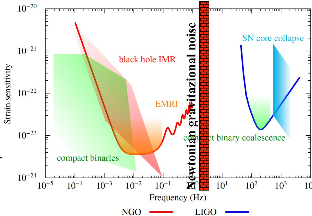
eLISA is sensitive at low frequencies (0.1 mHz – 1Hz) where ground based detectors cannot operate, due to Earth grav. noise
