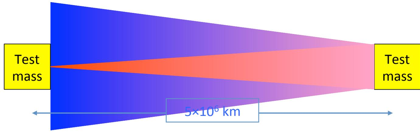
Power loss due to beam divergence makes interferometry by reflection impossible
