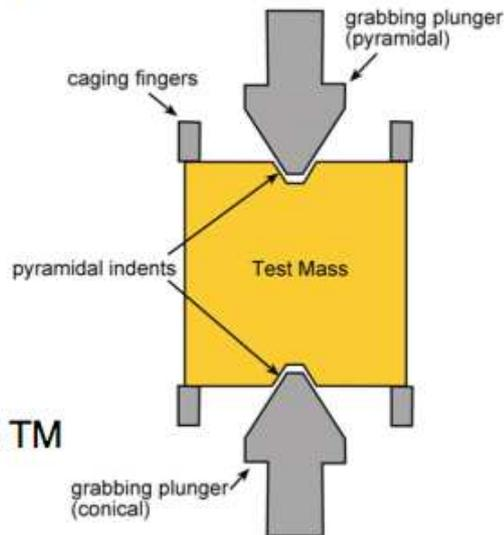
The Grabbing Positioning and Release Mechanism
