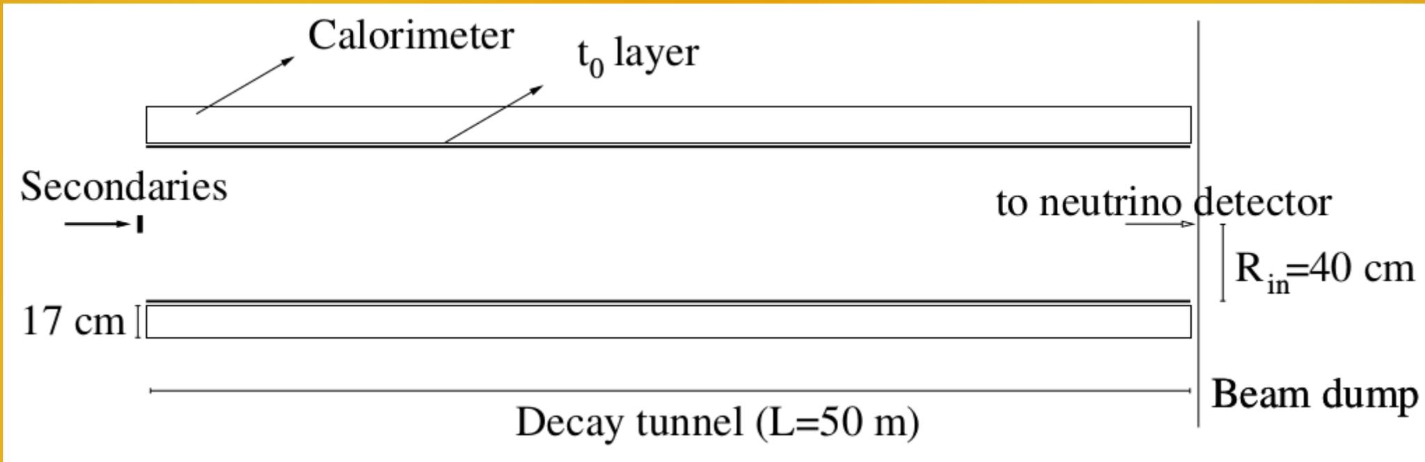
**$t_0$  layer:** a **pre-shower** providing absolute timing of arrival of the charged particle  $\rightarrow$  rejects neutral background ( $\pi^0$ ).
