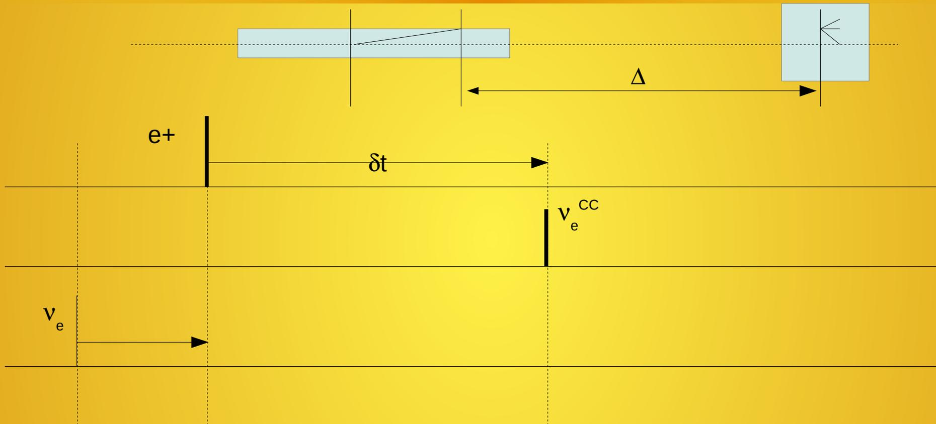
$\delta t \sim 50\text{-}100 \text{ m}/c = 170\text{-}330 \text{ ns}$ . The difference between the  $e^+$  and the  $\nu_e^{\text{CC}}$  time.
