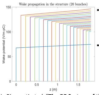
Longitudinal wake fields propagation inside the C-band accelerating cavities calculated at different instances corresponding to the  $n^{th}$ bunch arrive (n=0,1, ..., 20)
