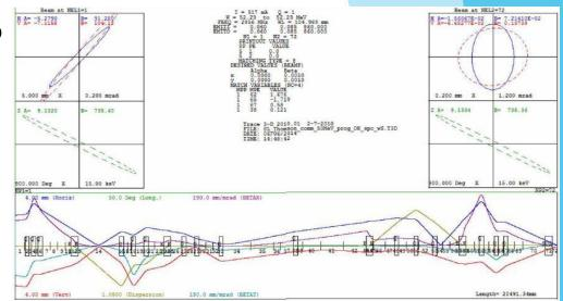
TRACE 3D simulation of Twiss parameters along the LINAC
