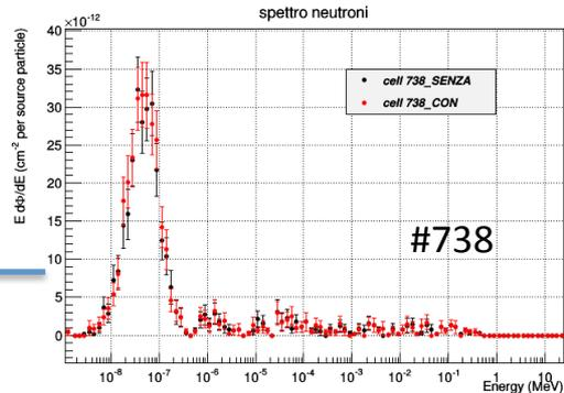
Neutron spectra in spheres of 20 cm radius with and without photoconverter
