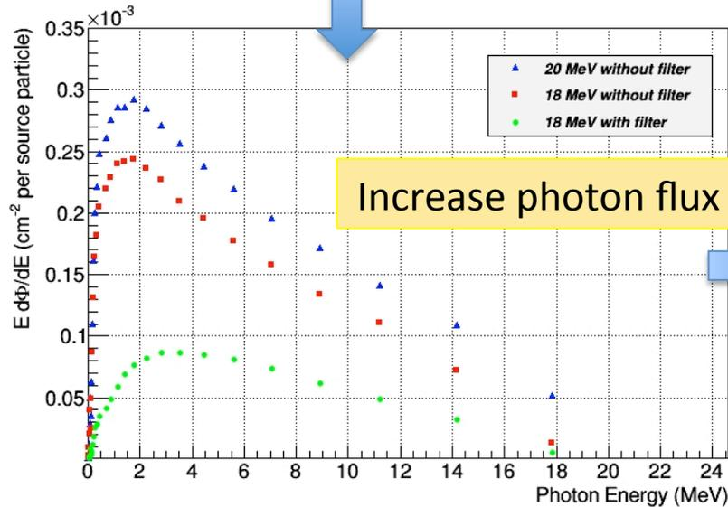
Photon spectra on a (20 x 20)cm<sup>2</sup> surface at 50 cm from the target
