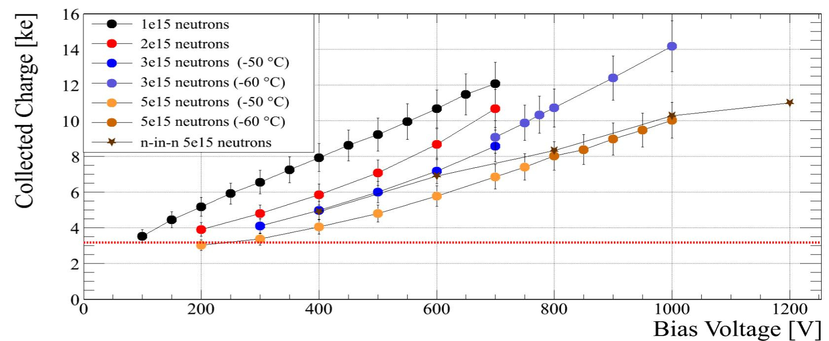
$V_{\text{bias}}$  not high enough to see charge-multiplication as observed in Micron devices for  $V_{\text{bias}} > 1600 \text{ V}$ ,  $> 1 \times 10^{15} \text{ n}_{\text{eq}}/\text{cm}^2$
