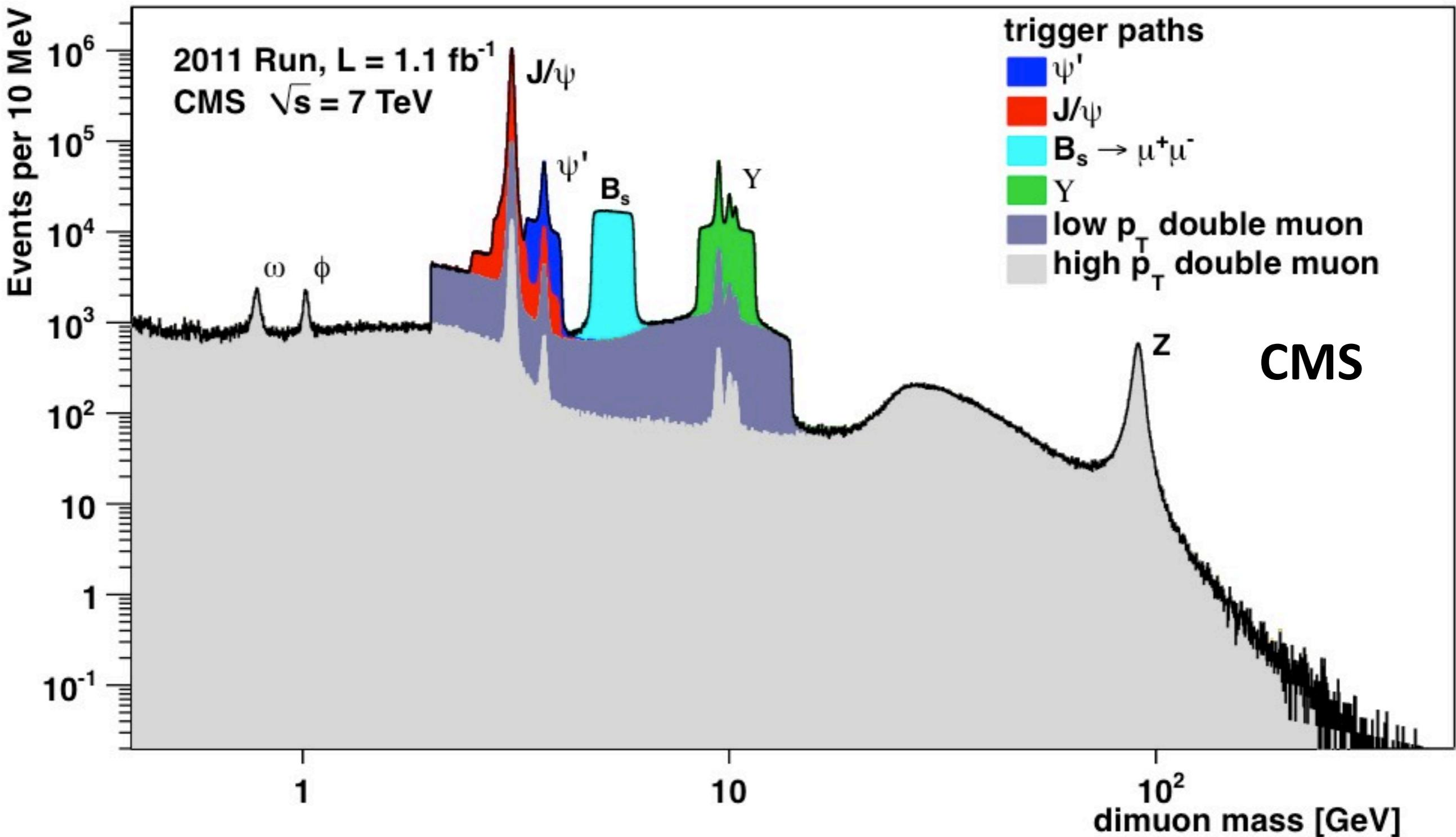
Dimuon mass distribution obtained from overlapping several trigger paths.
