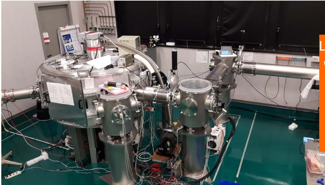
L3IA includes design and construction of a 12 MeV laser-driven proton beam line for diagnostics and beam handling applications. L3IA will be based on the ILIL laser installation at INO-CNR, currently undergoing 220 TW upgrade.
