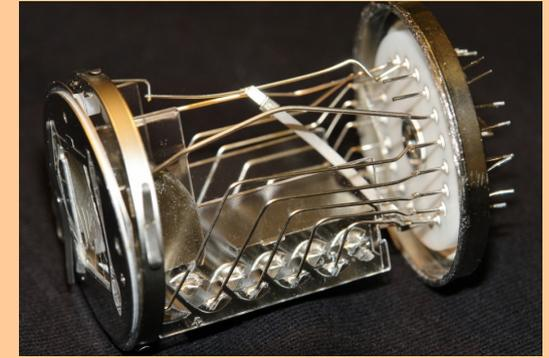
working with Hamamatsu to further improve the background of the R11410 PMTs for XENONnT
