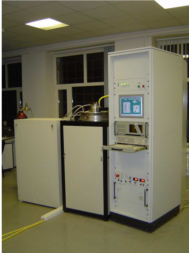
Laboratory microwave plasma chemical reactor STS-100 for growing diamond plates.
