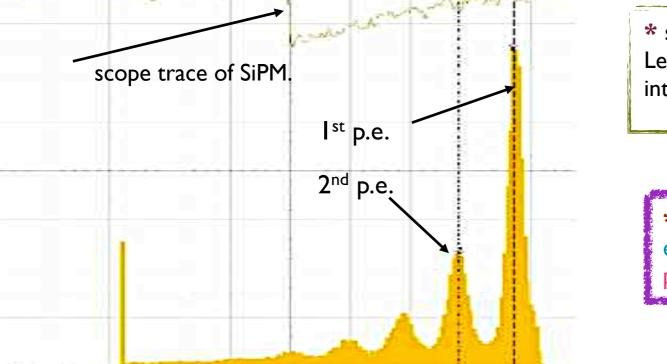
\* sample the thermal signal of the amplified SiPM with a Lecroy WaveRunner HRO 64Zi (12 bit - 2 GS/s) integrating the full signal charge.
