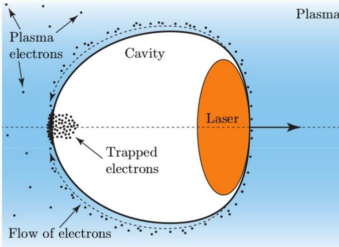
The bubble shape can be characterized by longitudinal and transverse radius. Basically, the longitudinal radius is the length of accelerating part of the wake. Simulation show that the longitudinal radius is linear in  $a_0$ . Threshold for self injection is represented in a  $(\gamma_0, a_0)$  plane, where  $\gamma_0$  is the wake velocity.
