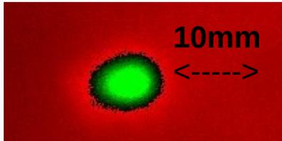
In some stable configuration  $\sim 15$  mrad circular electron beam has been observed. On the left a lanex picture (false color) 550 mm far from the gas-jet. Those result are obtained using **nitrogen** with backing pressure 4 bar which means  $1.9 \times 10^{18}$  N/Cm<sup>3</sup> density at gas-jet
