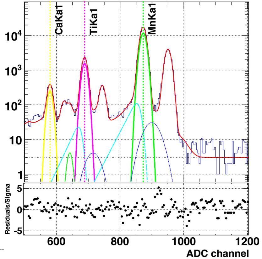
SDD Calibration: radioactive Source, X-ray tube
