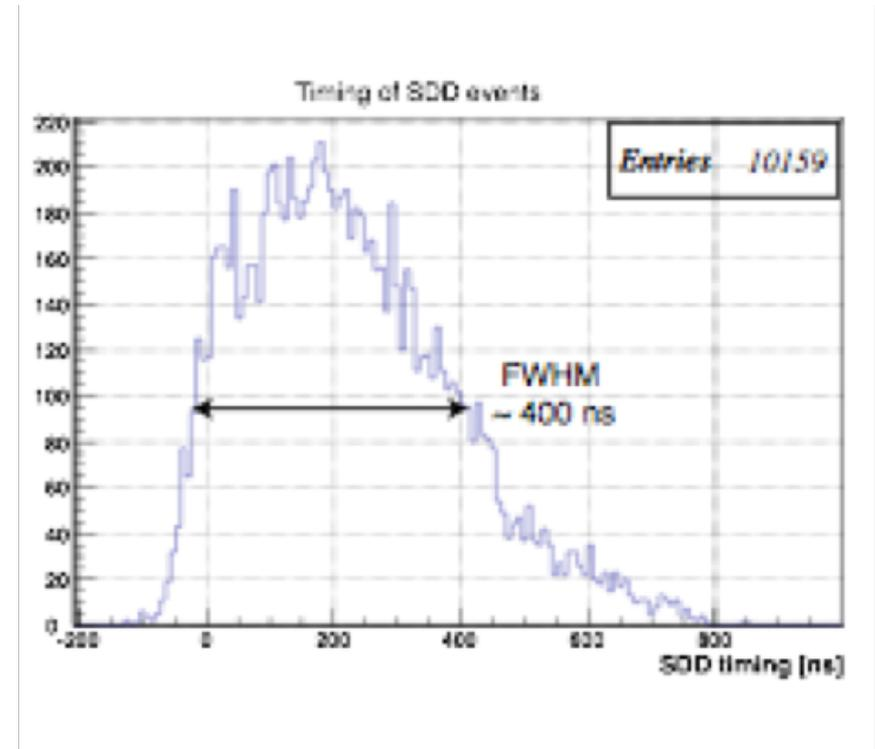
time resolution of SDDs from test setup measurement of cosmic rays
