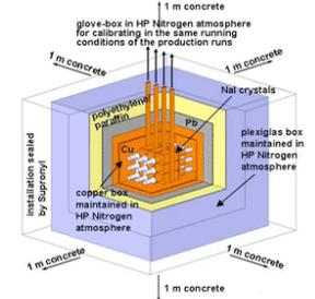
Simplified schema of ~100 kg Na(Tl) set-up
