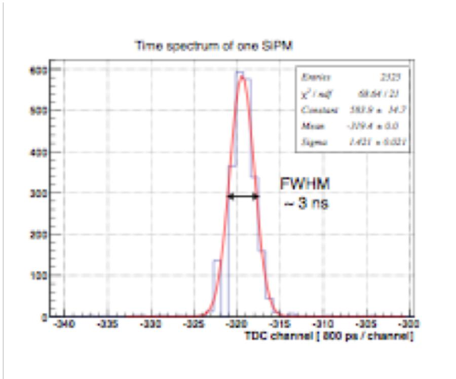
time resolution of scintillator from BTF measurement
