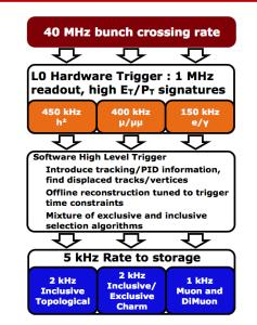
In Run I (2010-2012) of data taking the trigger reduces the input rate of 40 MHz to 2-5 kHz.
