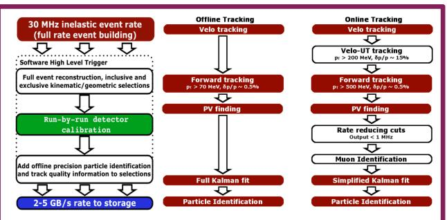
In the upcoming Upgrade run (>2020) the trigger system will be replaced by the software High Level Trigger which allows the full inelastic collision rate of 30 MHz to be processed. It will be possible for **the first time** in a hadron collider.
