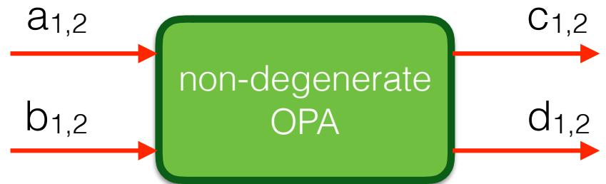
$$\begin{aligned} c_1 &= a_1 \cosh r + b_1 \sinh r \\ c_2 &= a_2 \cosh r - b_2 \sinh r \\ d_1 &= b_1 \cosh r + a_1 \sinh r \\ d_2 &= b_2 \cosh r - a_2 \sinh r \end{aligned}$$
