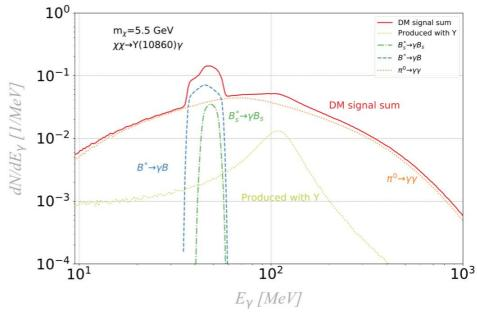
Example of the expected gamma-ray spectrum for DM annihilation into charm quarks, with a DM mass mx just above the kinematic threshold to produce Dmesons.
