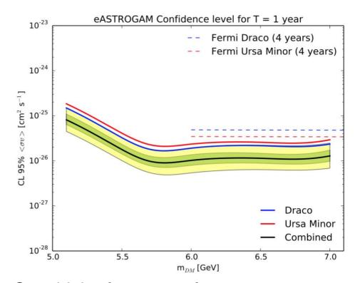
Sensitivity for < σv > from observation of the classical dwarf galaxy Draco and Ursa Minor for self-annihilation channel bb for 1 yr of effective exposure compared to 4 years of Fermi LAT in survey mode.
