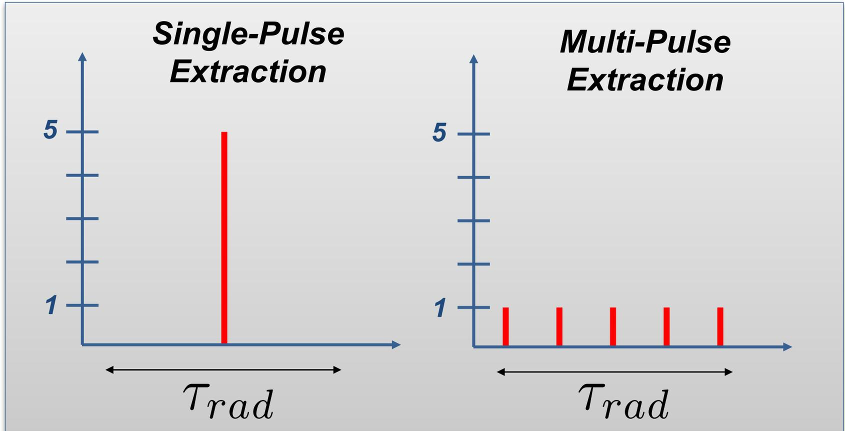
Multi-pulse extraction reduces the effective fluence in the laser system and therefore moves the operating point into a manageable regime for low cross-section materials
