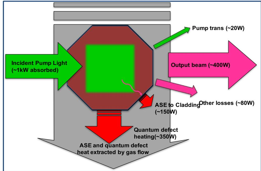
The short gain lifetime and the large quantum defect make Ti:Sapphire drives the cost of the pump laser and makes it an unattractive HAP laser medium
