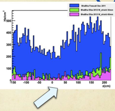
Significant reduction of the neutron rate on Barrel LO from 450 Hz/cm<sup>2</sup> to ~50 Hz/cm<sup>2</sup>: 1 order of magnitude less
