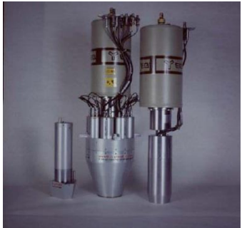
GASP coaxial HPGe det. Of GALILEO With new digital electronics:
