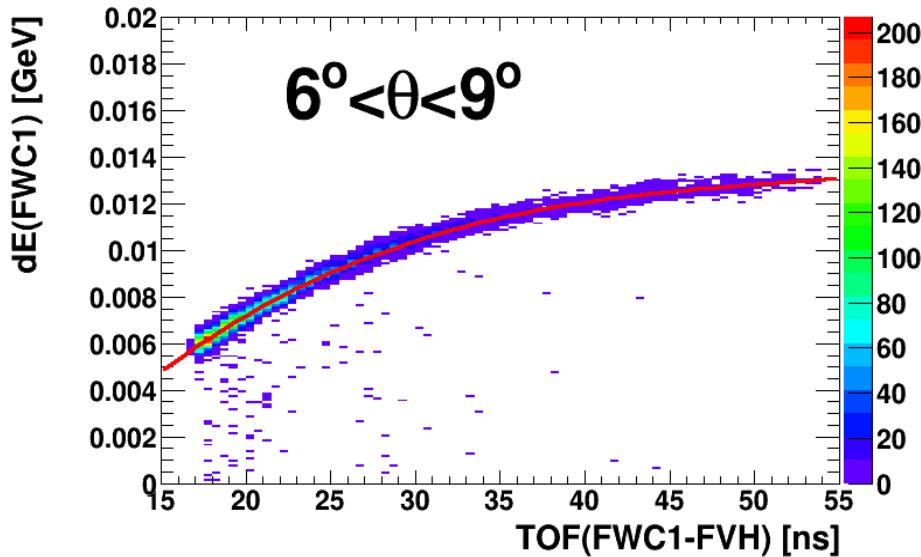
**Data:**  $dE$  [channels] vs ToF [ns]  $\rightarrow dE_{\text{ch}}(\text{ToF})$
