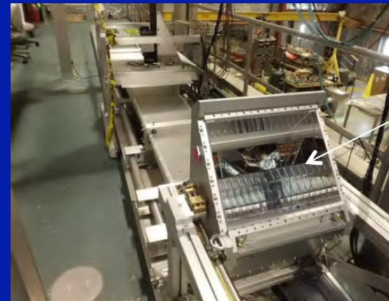
**Fabrication of the FDIRC prototype optics and mechanics successfully finished !!!**
