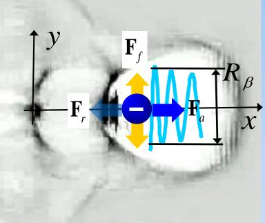
When the force of radiative friction is disregarded, the first two equations are equivalent to the equation of linear oscillator with a slowly varying frequency.
