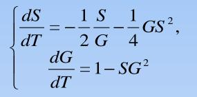
As G > 0 and S > 0 then dS/dt < 0 and the amplitude of the betatron oscillations always decreases with time. This means that for arbitrary electron energy the betatron oscillation amplitude will be small enough at a certain instance of time to be radiation reaction force less than the accelerating force.
