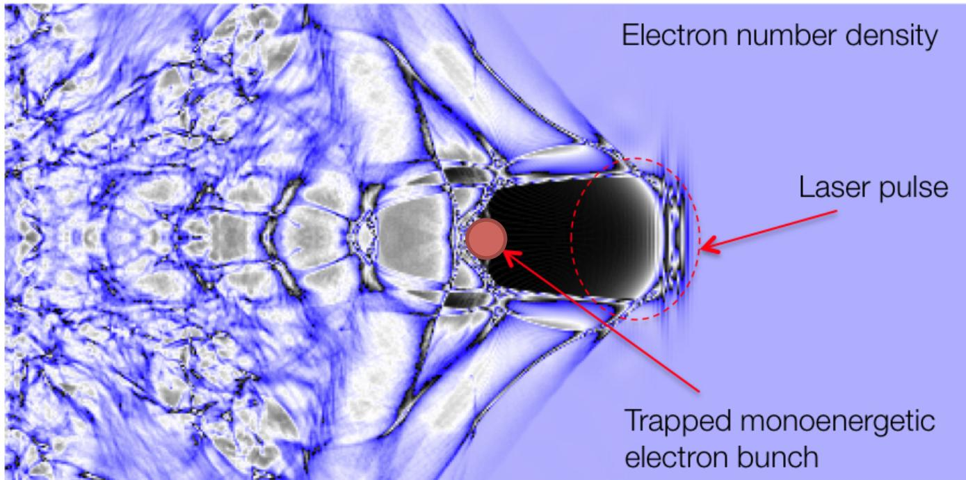
Electrons accelerated by the linac injected with the right phase on the creast of the wakefield to be further accelerated.
