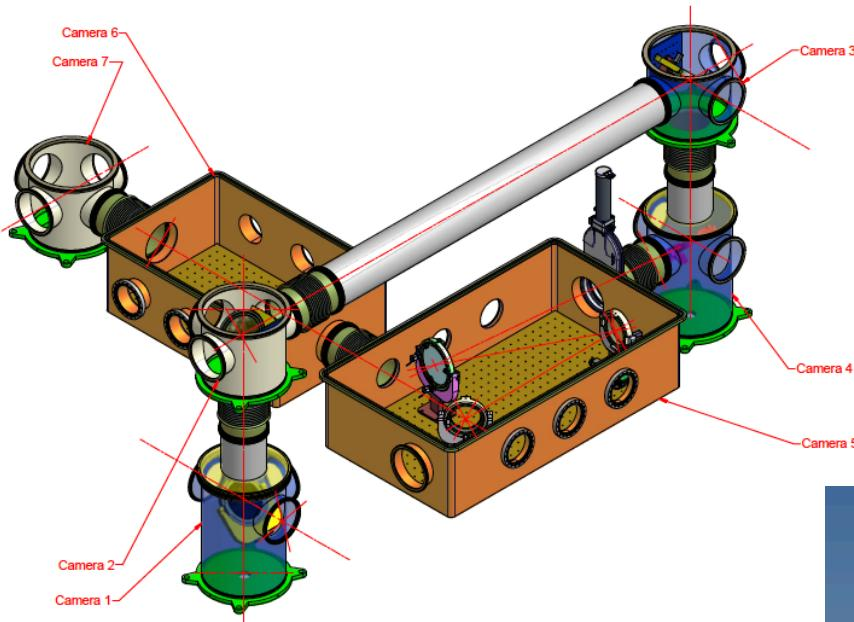
Design of the vacuum chamber for the laser transport.
