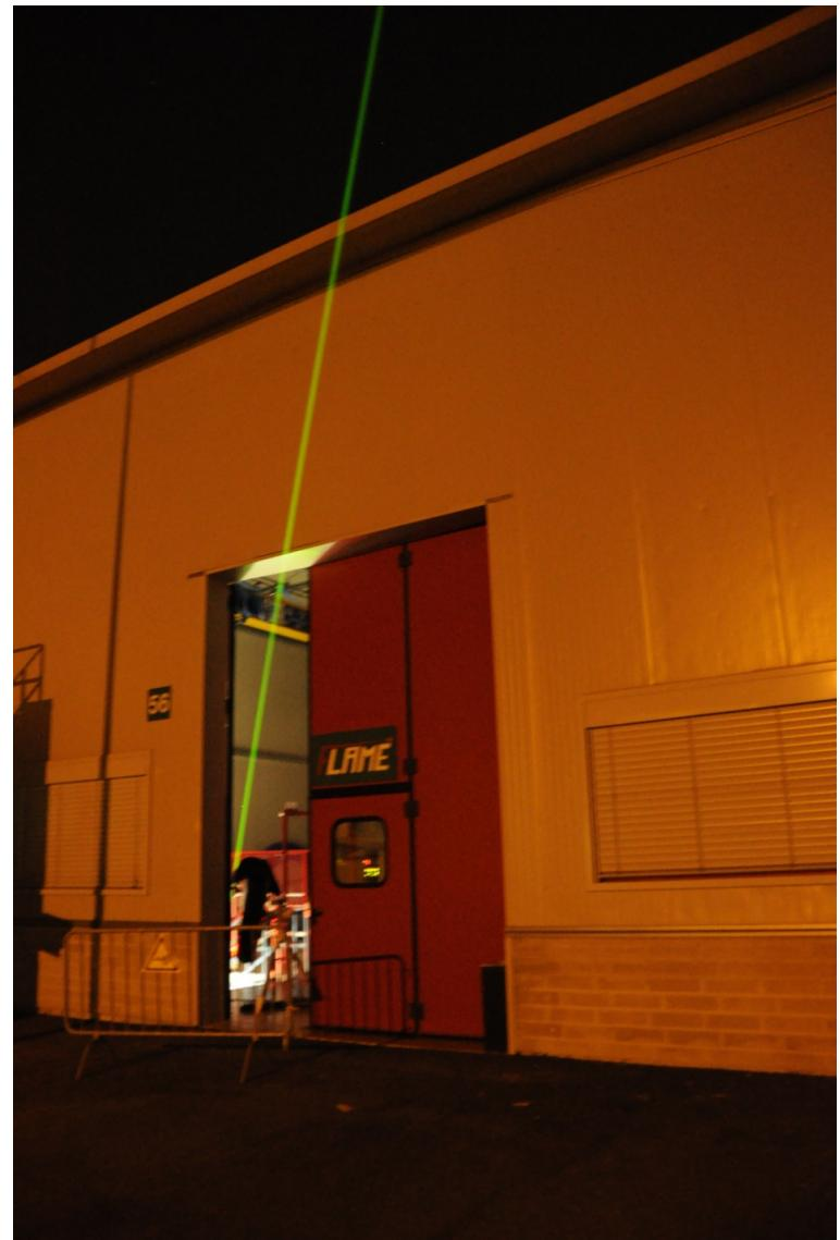
Backscattering light (LIDAR signal) from the plasma filaments.
