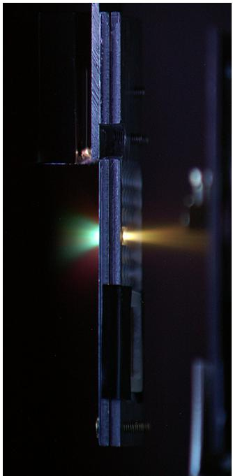
The principle of work of proton acceleration by thin metal target (TNSA) is to focus a high intensity laser on a thin metal target in order to generate a plasma on the surface of the target. This process generates a burst of MeV fast electrons contained in the target (by the very strong electrostatic field generated by charge separation). These some field also act to accelerate protons at the target surface out into the vacuum.
