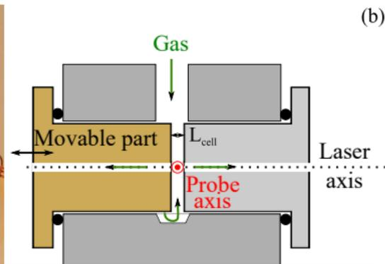
The mean density inside the gas cell was first experimentally characterized.
